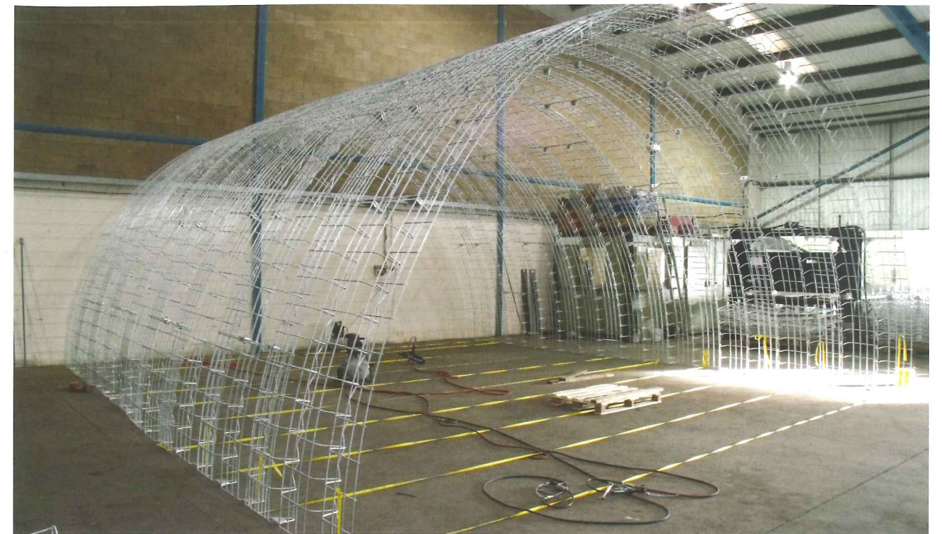
Above: RamArch is a system developed for Network Rail by Innovative Support Systems
