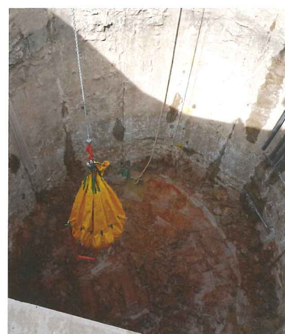
Below: A jib crane is assembled on site, which was an unusual challenge and is then tested with water bags to simulate the load of a man rider
