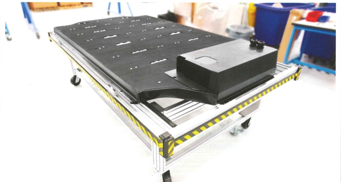
Below: Figure 7, Tesla Model S lithium-ion battery pack 9
