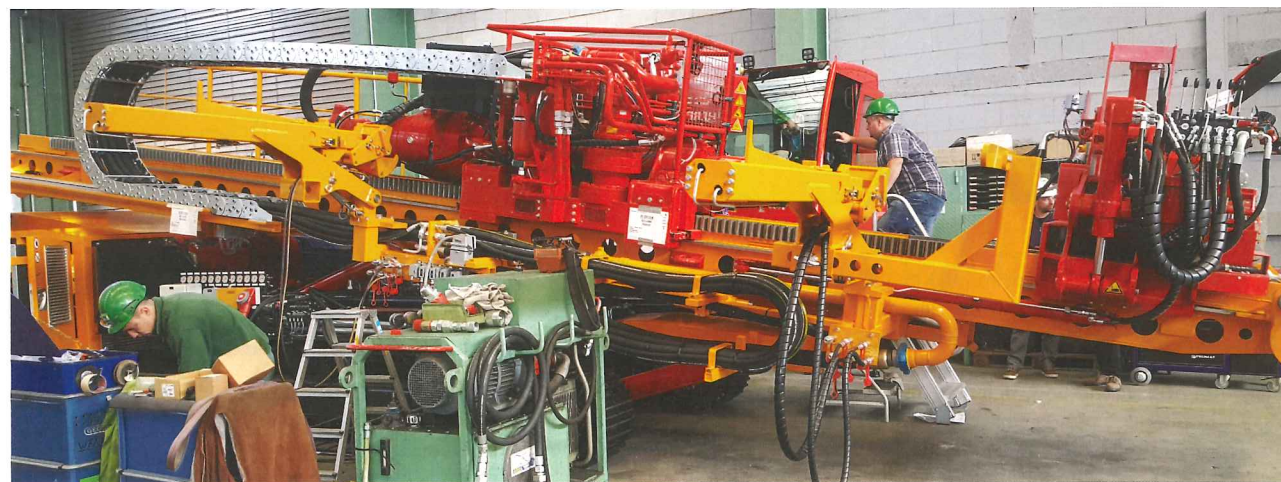
Below: A horizontal directional drilling rig
