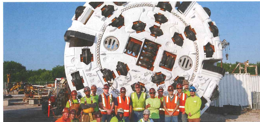
The S-K JV stands proudly in front of the 6.2m cutterhead
