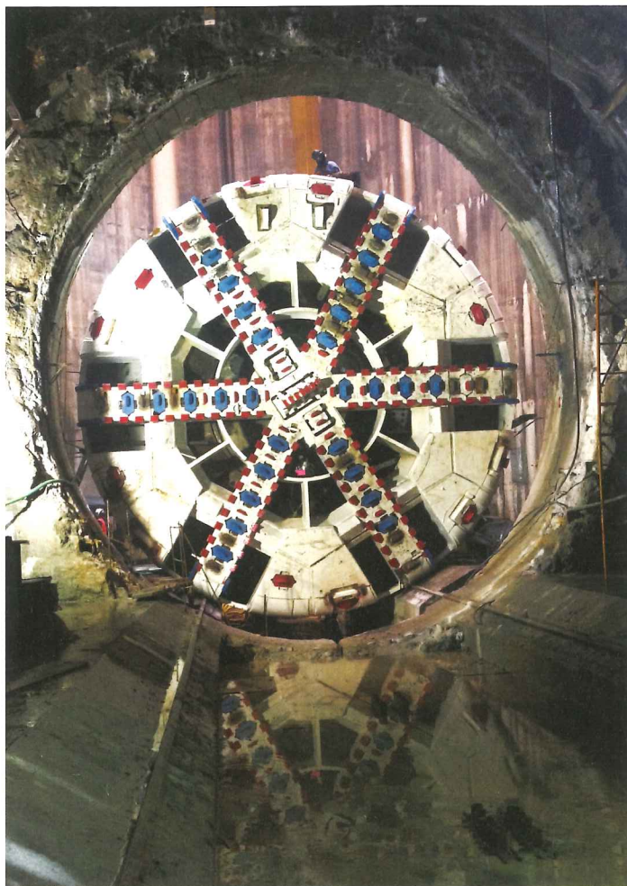
Above (left): The TBM on the Emisor Oriente project was installed with carbide bits rather than disc cutters
