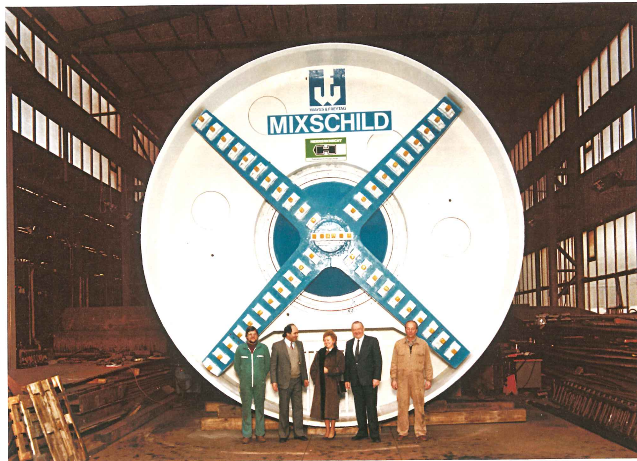
Above: In 1985 Herrenknecht works with Wayss & Freytag to produce the first large diameter (6m) Mixshields. This one worked on the 6.2km HERA particle accelerator
