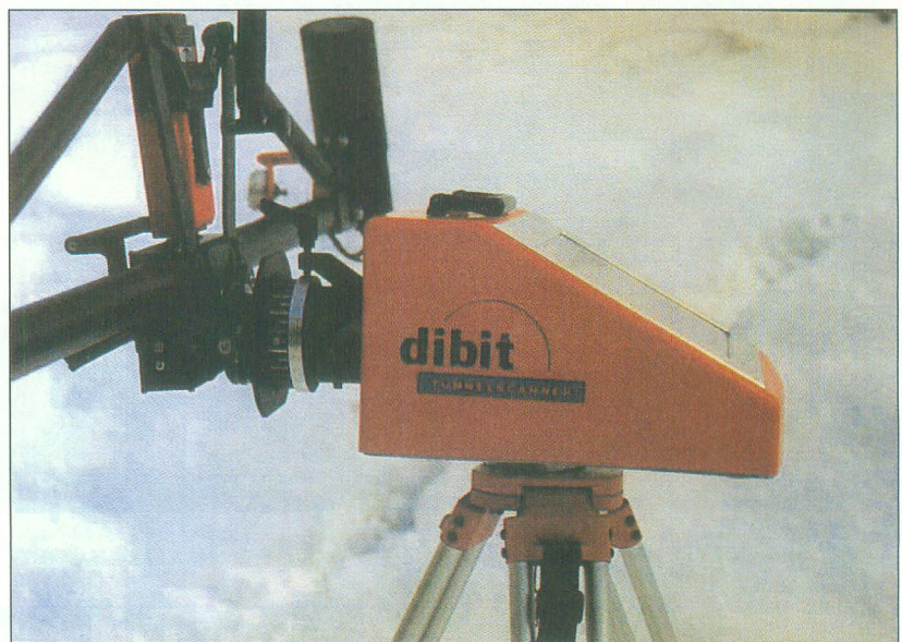
DIBIT-Recording module field computer with camera frame on tripod
