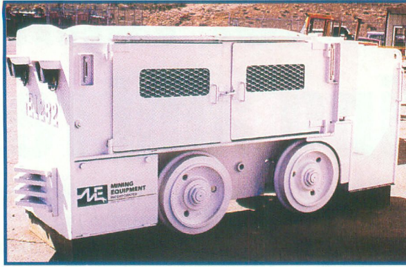
A Clayton 10-ton diesel locomotive, powered by a Deutz Model F6L912W engine
