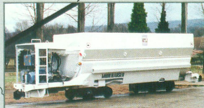
UNICAR, 10 m 3 , for TUNNEL WESTERSCHELDE NL
