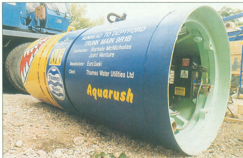
The freshly named 'Aqurush' Iseki 1450mm o.d. Unclemole ready for its first drive
