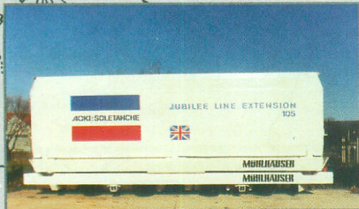
floorshaftcar, 12 m 3 , for JUBILEE LINE EXTENSION GB
