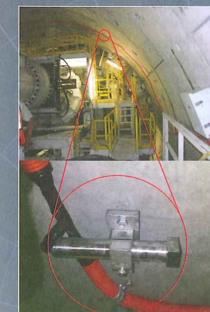
Typical installation of the RST Profile Monitoring System for Tunnel Concrete Segments with an RST flexDAQ Datalogger System.
