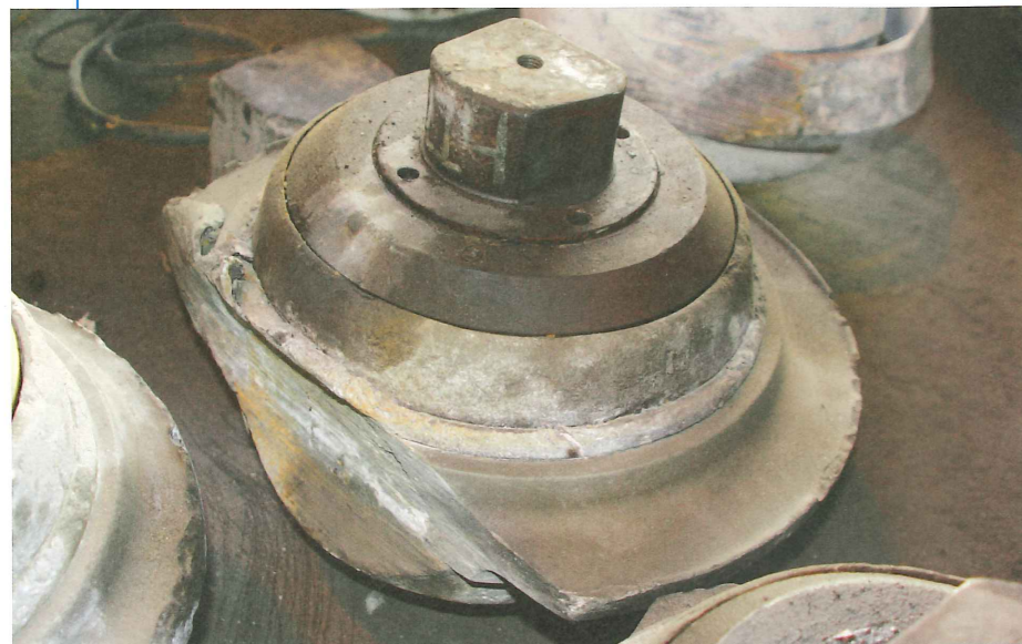
Above: A cutter disc unevenly worn after becoming stuck on the hard rock
