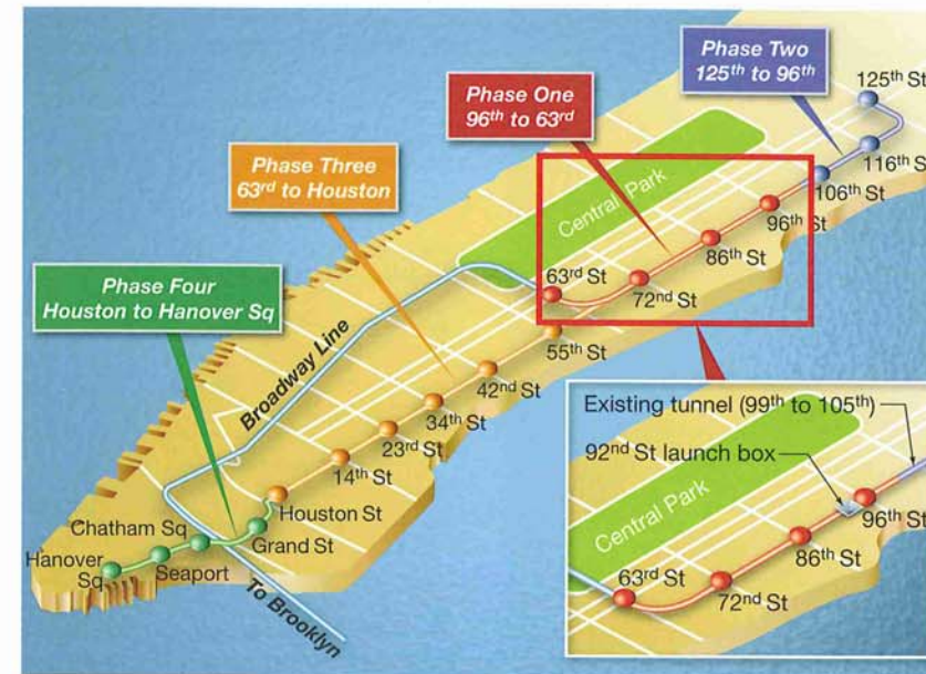
Above: Figure 1 - The Second Avenue Subway will be built in four phases; Phase One (inset) is schedule to be operational by 2016
