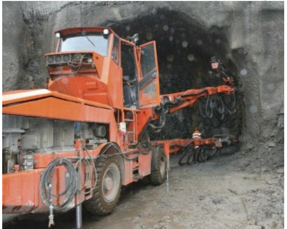
Above: A drive from Hedinsfjordur valley to blast Olafs from the opposite direction started in May 2008 but at a shallower slope than first planned to give longer distance uphill and avoid any downhill grade risk with groundwater before breakthrough underground
