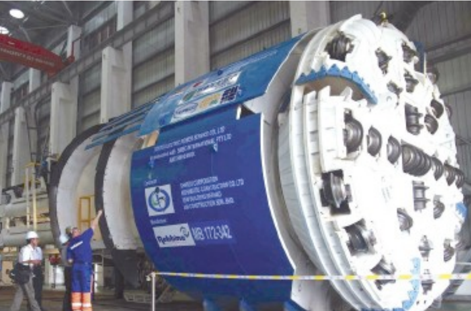
Far left: The Pahang Selangor Tunnel, Malaysia's largest infrastructure project, required the simultaneous assembly of three 5.2m TBMs in Shanghai and required the support of local firm Jui Ba Left: Assembly of the first of the TBMs was completed in early July 2010.
