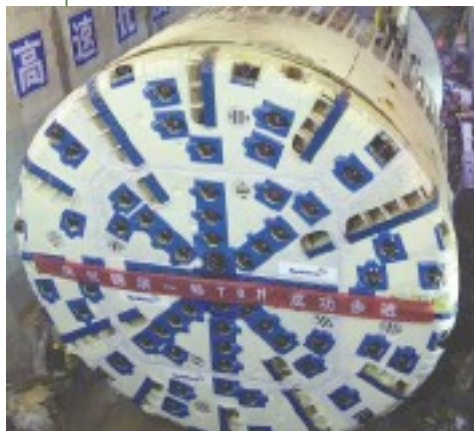
Left: The 12.43 m Robbins TBM was launched in September 2008, following an onsite assembly that took just three months
