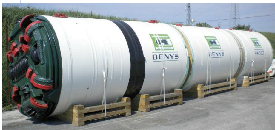
Below: Denys is using four Herrenknecht AVNs on the micro-tunnelling contract
