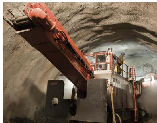
Below, right: Rear view of the MT520 showing truck-loading conveyor
