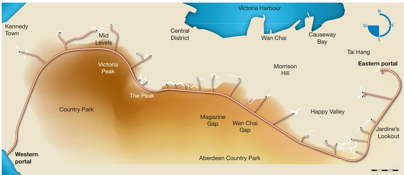
Above: The tunnel alignment picks up intake adits in the hill side
