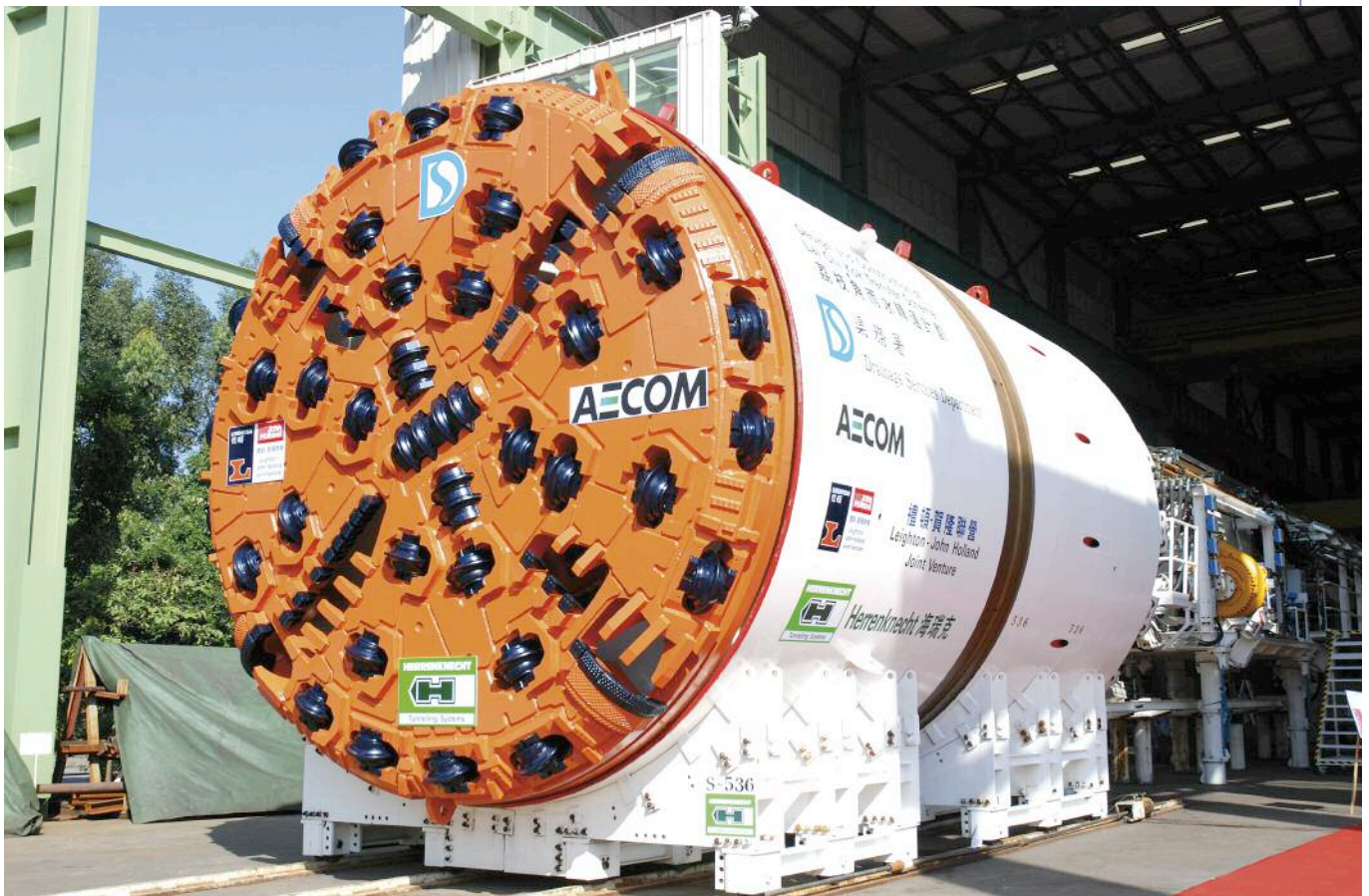
Below: The 5.72m TBM at Herrenknecht’s factory in China
