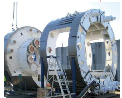
Above: The 6.13m diameter DSU TBM will bore the 14km under the Himalaya chain
