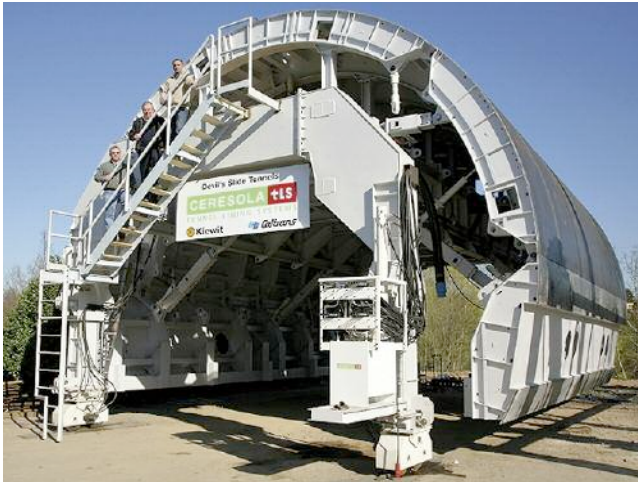
Above: Longitudinal section through tunnel alignment showing main geological features. The varying surface profile are over the two centerlines of the bores. Left: The Ceresola travelling formwork before delivery to the site (Photo: Ceresola)
