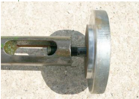
Above left: Tracto-Technik QuickLock bursting rods and anchor plate; Left middle: Adapted bursting rod with bolt connector and anchor plate; Left bottom: Anchor plate connector and a sheared bolt; Above right: Demonstration attendees discuss the issues
