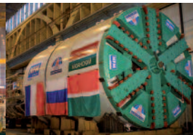
Soft ground TBM
