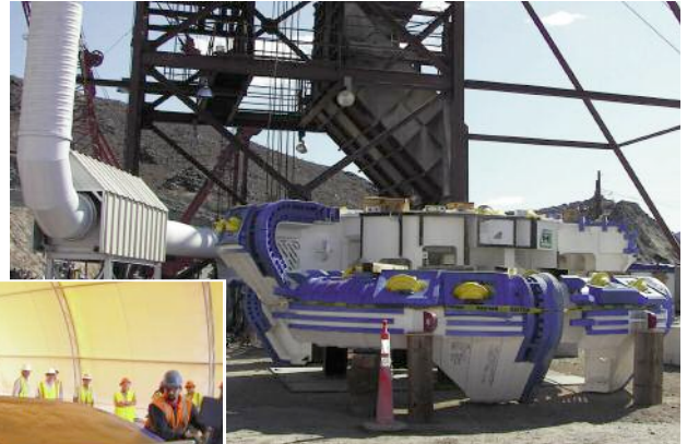
Above: VTC's state-of-the-art 23.5ft diameter Herrenknecht Mixshield TBM begins to arrive on site Left: Segment manufacture underway
