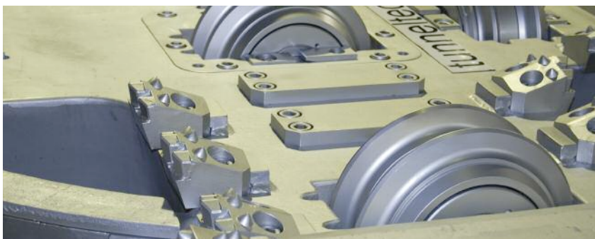
Right: Part of a dual-function 2,26m-diameter TunnelTec rock cutterhead delivered last year to contractor Dibco of Toronto. It features both fixed and disc cutters and can be converted to soft-ground use. Its first project was for a siphon sewer in Calgary.
