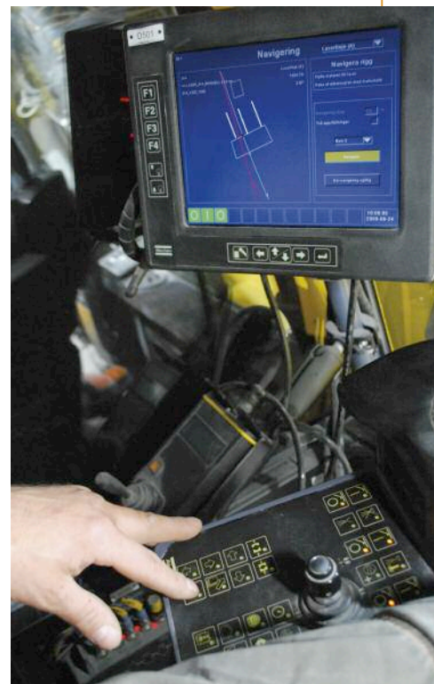
Below, left: Fig 3 – The system then finds the position of the rig in the tunnel by locating reference prisms mounted on the tunnel walls
