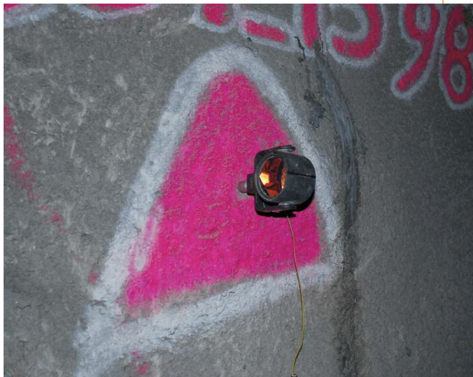
Below, left: Fig 3 – The system then finds the position of the rig in the tunnel by locating reference prisms mounted on the tunnel walls
