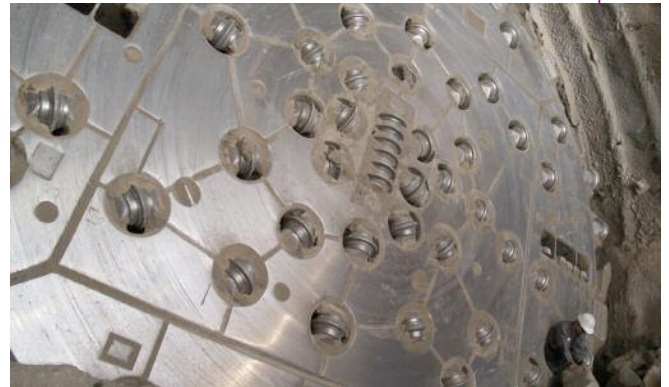
Above left: Breakthrough of an 8.16-m Wirth EPB TBM equipped with TunnelTec tools on the Castellanza metro project, Italy. The cutterhead is equipped with both static rippers and scrapers and disc cutters with carbide bullet inserts. Right: Disc cutters shown on the cutterhead of a 9.90m-diameter NFM Technologies TBM on completion of 1140m in a single month for the Madrid-Gijón high-speed railway route
