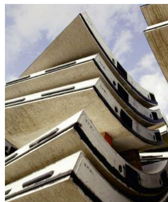
Below left: Precast segments with PVC liner are being used to prevent corrosion; Below right: The Robbins EPB has active articulation to tackle 1,300ft (400m) radius curves without segment deformation
