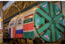
Soft ground TBM
