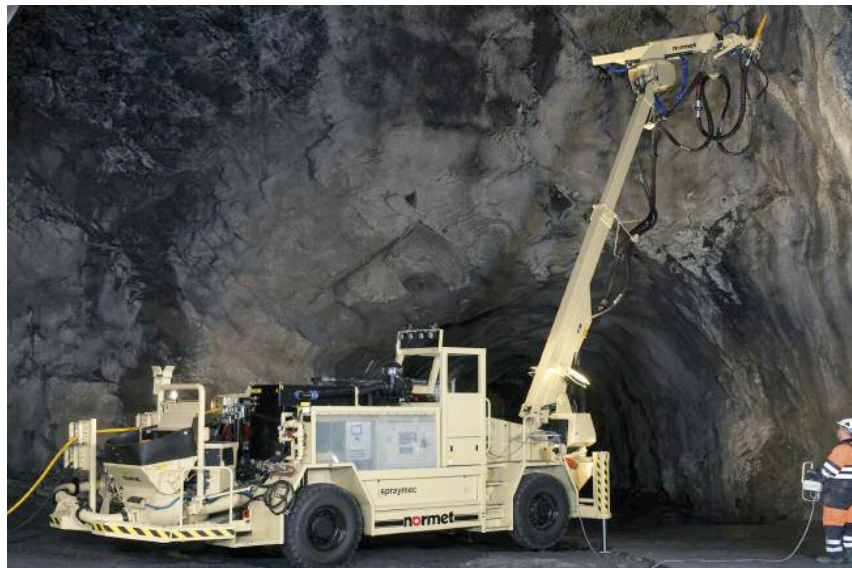
Below: The second largest rig in the Normet range, the Spraymec 7110 WPC can cover a wide variety of tunnel sections from a rigid carrier with 4-wheel steering
