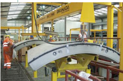
Left: Fitting gaskets to segments at the Morgan Est Ridham plant
