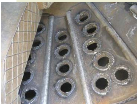
Below (L-R): The AVN's narrowed cutterhead ports; Jacking setup in one of the secant pile shafts; View of face during free air intervention
