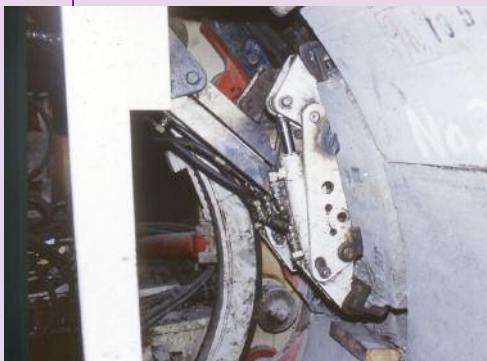
Above: The open face backhoe for the Three Valleys Water Company tunnel Left: The original segment erector either dropped or spalled segments
