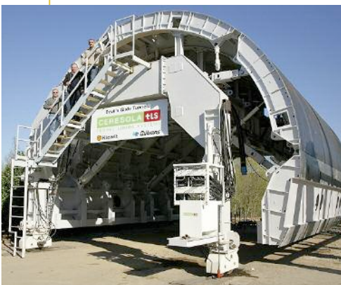
Left: Ceresola TLS recently supplied two bespoke self-travelling forms to the Kiewit Pacific JV for the Devil's Slide project, in California, USA
