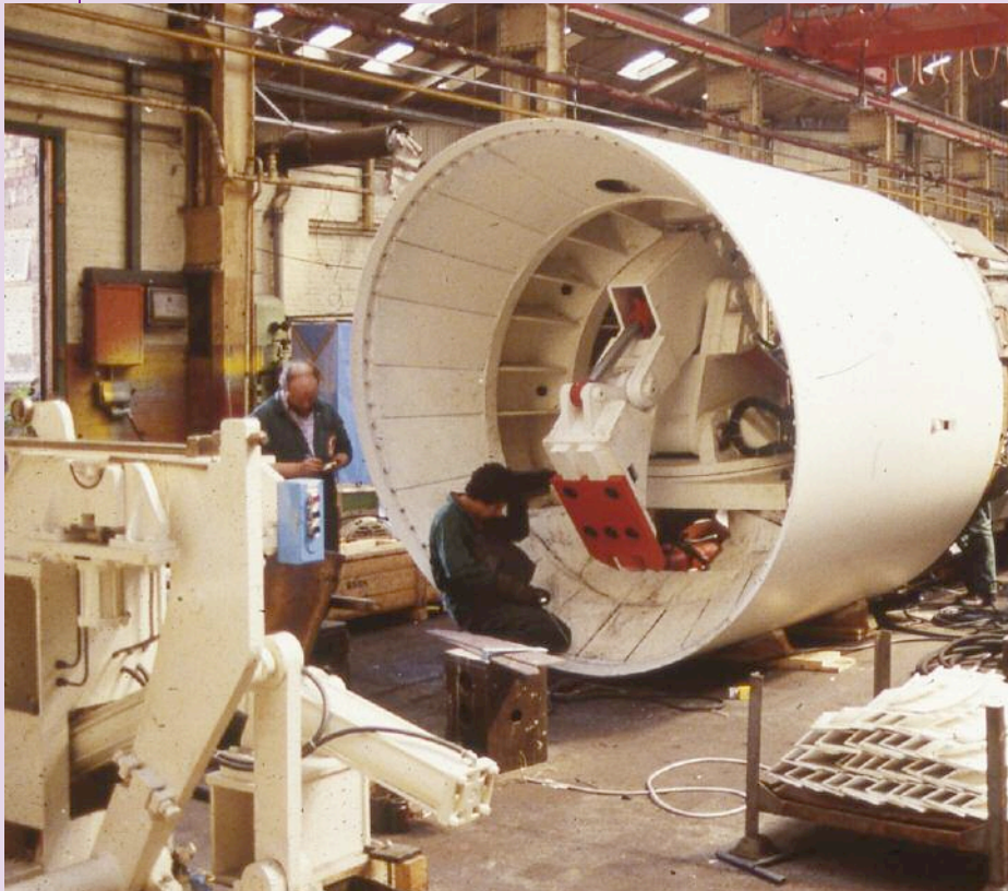
Above: The open face backhoe for the Three Valleys Water Company tunnel Left: The original segment erector either dropped or spalled segments
