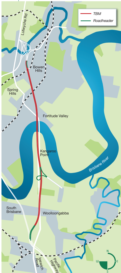
Above: Plan map of the alignment of Brisbane's north south road tunnel
