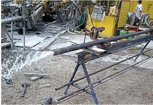
Above, from left to right: DeviDrill hydraulic test before running in hole; DeviDrill orientation; Dogleg eccentric housing
