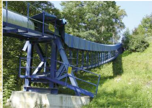
Left and below: The ability of conveyor systems to traverse steep valley sides, rivers and roads, can offer big advantages for large-scale projects such as the Jinping II HEP
