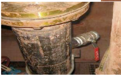
Below and right: The balancing pipes in the TBM – for flushing provision
