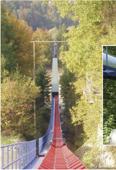
Left and below: The ability of conveyor systems to traverse steep valley sides, rivers and roads, can offer big advantages for large-scale projects such as the Jinping II HEP
