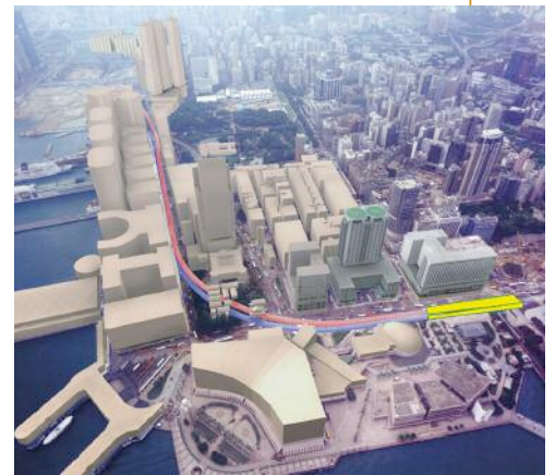
Above: Alignment of the drives, as seen from the southern East Tsim Sha Tsui Station interface
