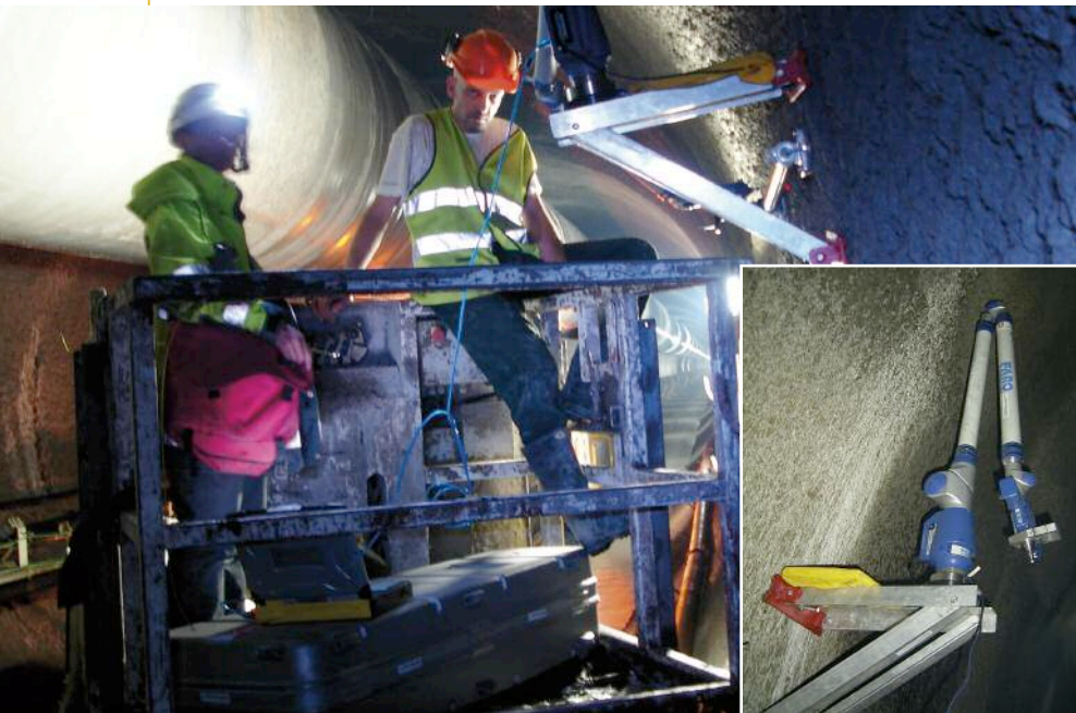
Above: Following the visual inspection to pre-categorise the rocks into roughness classes, about 10% of inspection sites were scanned by wall-mounted laser
