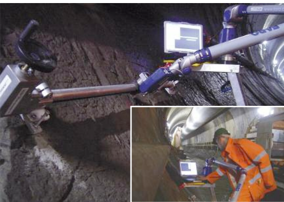
Below: The laser scanned vertically-separated strips of wall surface
