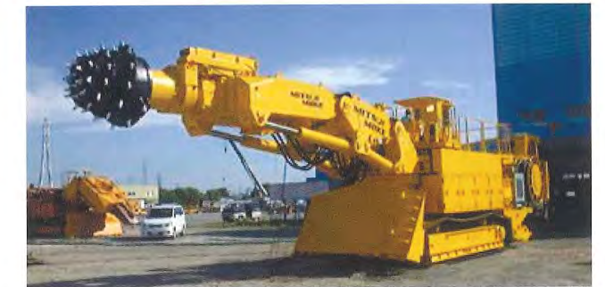
Large roadheader (350 kW)
