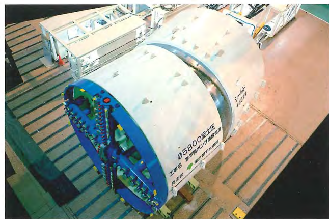
Articulated structure of the shield machine
