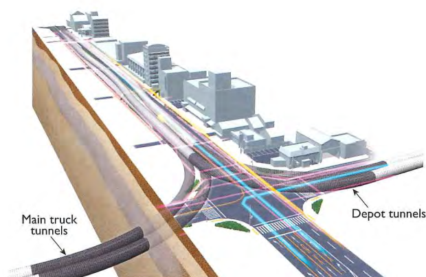
Schematic view of the Osaka subway No.8 line
