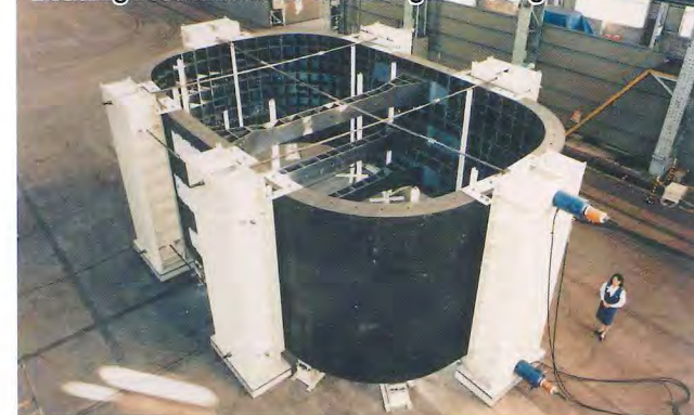
Loading Test on Ductile Steel Segment Rings
