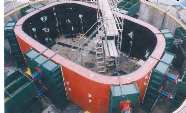
Loading Test on Sandwich Type Composite Segment Rings
