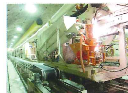
Photo 2 Fiber mortar spraying equipment mounted on TBM
