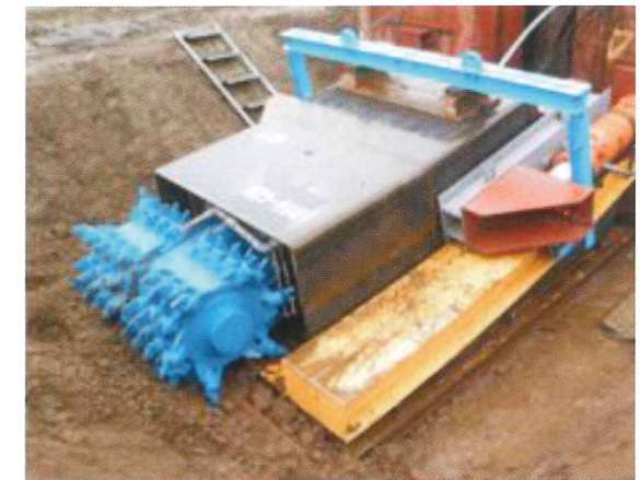
Photo 1 Boring machine (twin header)
