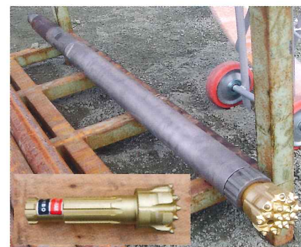
Photo 2 Detail of drill bit
