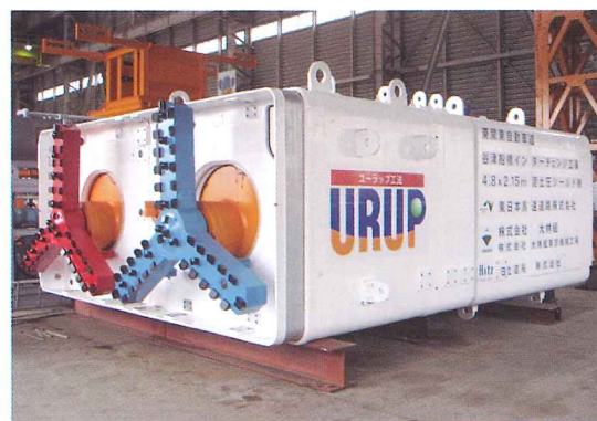
Photo 1 Closed type high, density slurry shield method
