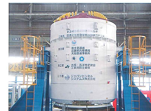
Photo Upward shield machine
