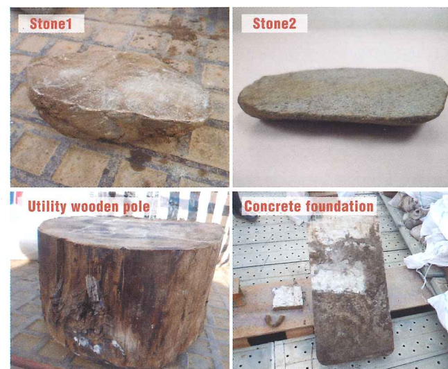
Fig. 4 Obstacles cut and removed
