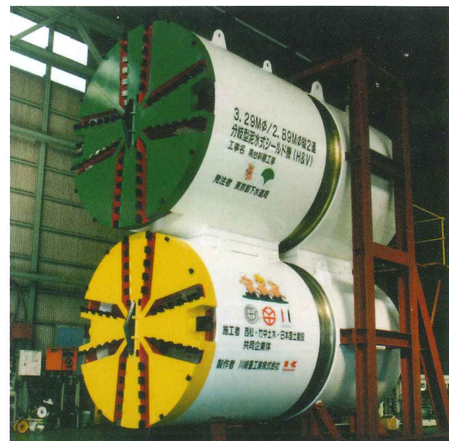
Photo 2 Twin multi-head shield for stacked tunnels (upper: φ 3,290 mm, lower: φ 2,890 mm) (Minami-dai sewer main)
