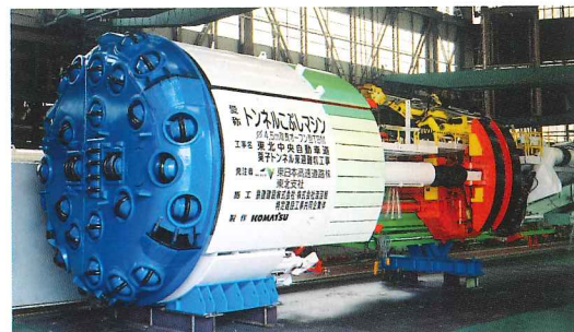
Photo 1 Main system of the TBM 4.5 m diam.
