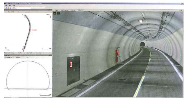
Below: Figure 4, True colour rendered scan model of a road tunnel
