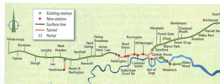
Below: Figure 1, Overview of the Crossrail project
