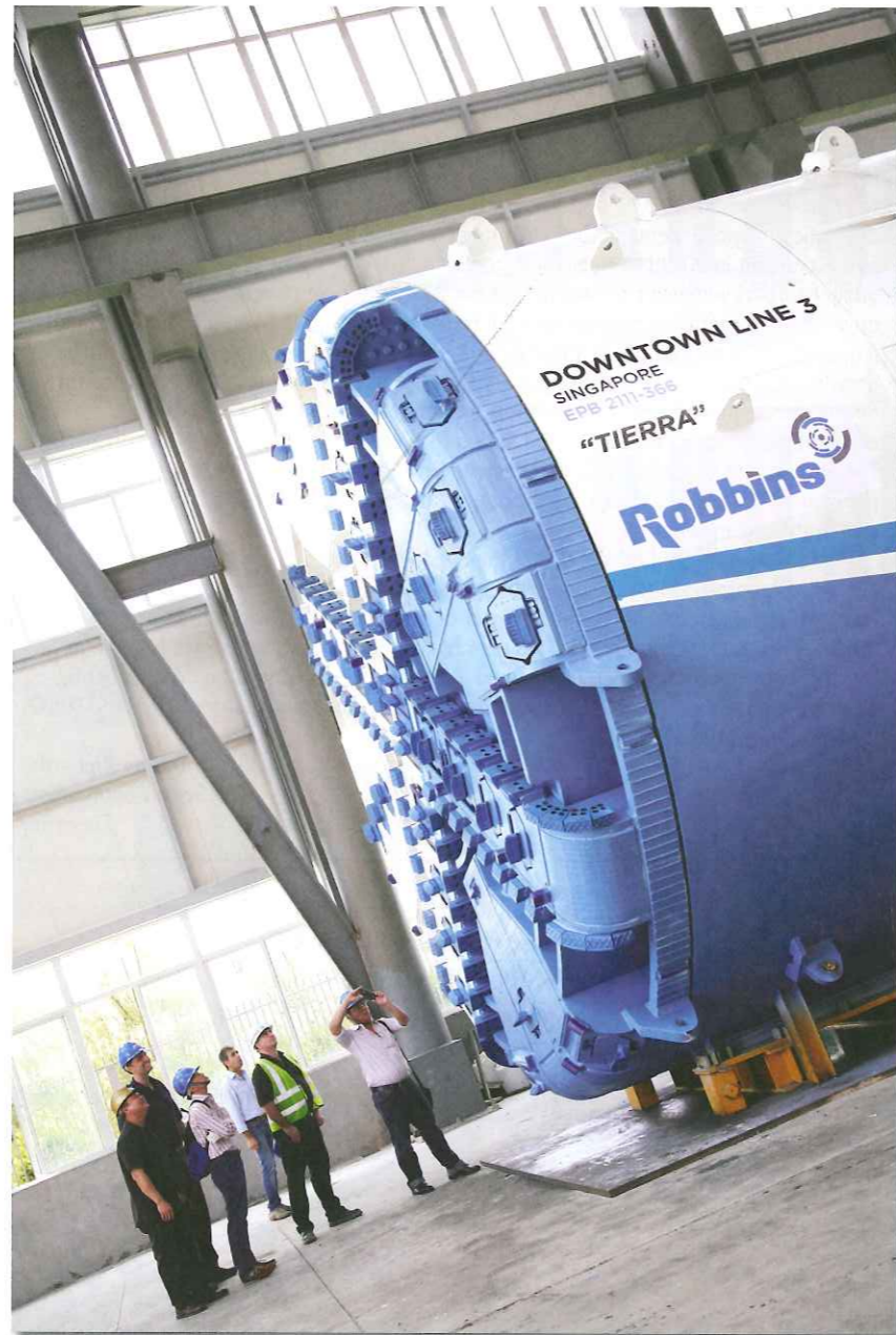
Above: Mixed ground conditions ranging from clay to mudstone, sandstone and boulder fields dictated the use of mixed ground EPBs on many of the tunnels.
