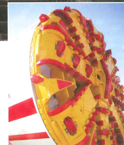
Above: The machine being lowered down the shaft to bore the second metro line Right: Herrenknecht manufactured the four EPBMs for the project. The machines have a diameter of 6.3m, giving a finished tunnel i.d. of 5.4m
