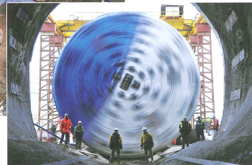
Above: A 10m diameter Robbins double shield TBM will line its headrace tunnel with segments for the first 3km, switching to ring beams, rock bolts, and wire mesh in more stable ground
