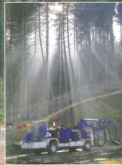
Left: Entrance to the twin bore Hindhead tunnel, which was constructed using sequential excavation and SCL; Inset: The BASF Meyco shotcreting rig
