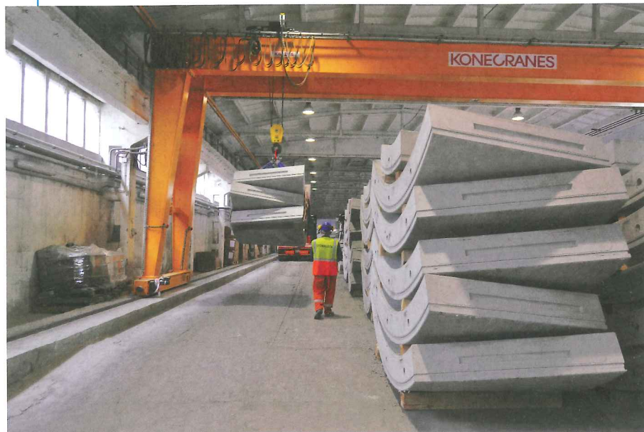
Above: Segment stacking showing the five plus key arrangement
