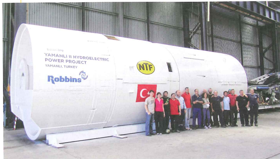
Above: The Robbins crew and contractor NTF stand in front of the 4.3m Robbins double shield for the Yamanli II HEPP, currently being assembled in Italy
