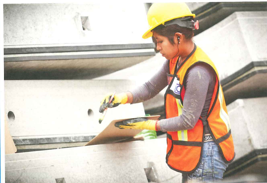
Above: Custom segments were manufactured 24 hours per day by contractor ICA, then trucked daily to the small station sites
