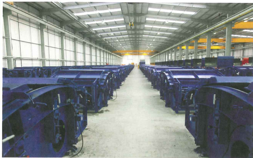
Above: Some 213 CBE moulds are needed for segment production by the BFK JV
