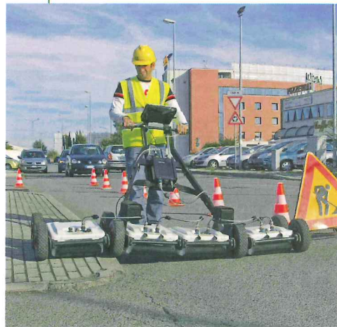
Left: A ground penetrating radar instrument used for detecting buried services, objects, etc in a highway (Photo: European GPR Assoc)
