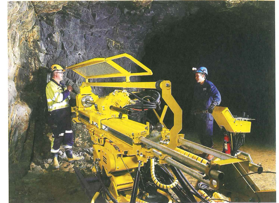
Above: Atlas Copco's Diamec U6 underground core drilling rig that can be easily positioned for any direction
