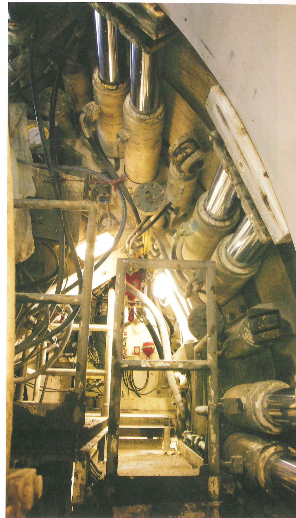
Right: The machine is propelled by 16 pairs of hydraulic cylinders
