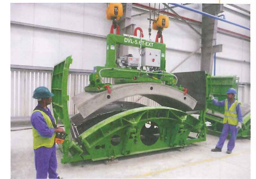
Left: A concrete segment factory supplies Impregilo and can produce 42 segments per day; Above: Herrenknecht Formwork has manufactured the moulds
