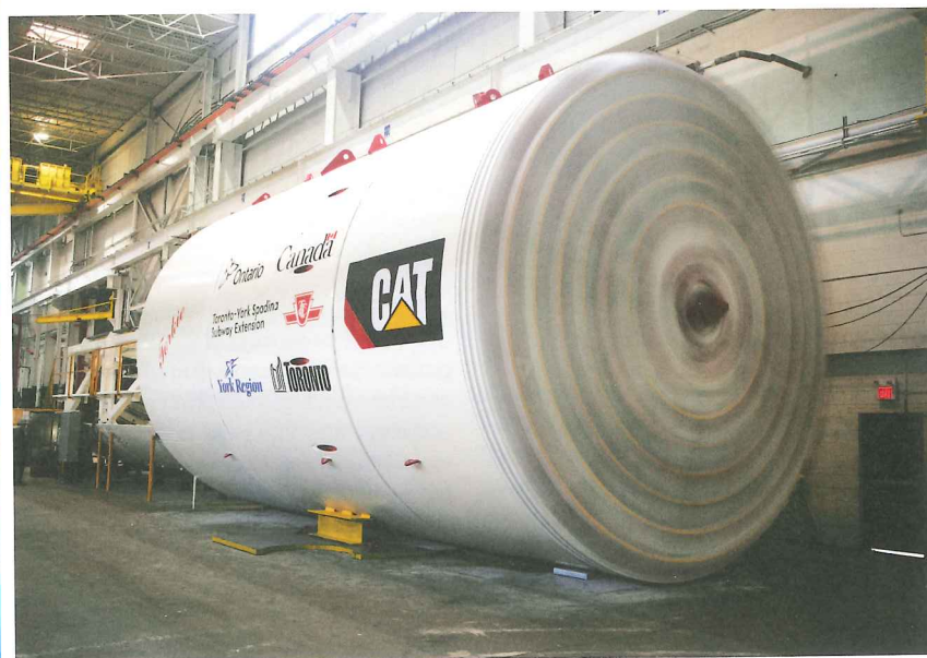
Below: One of the TBMs being manufactured for the Crosstown line
