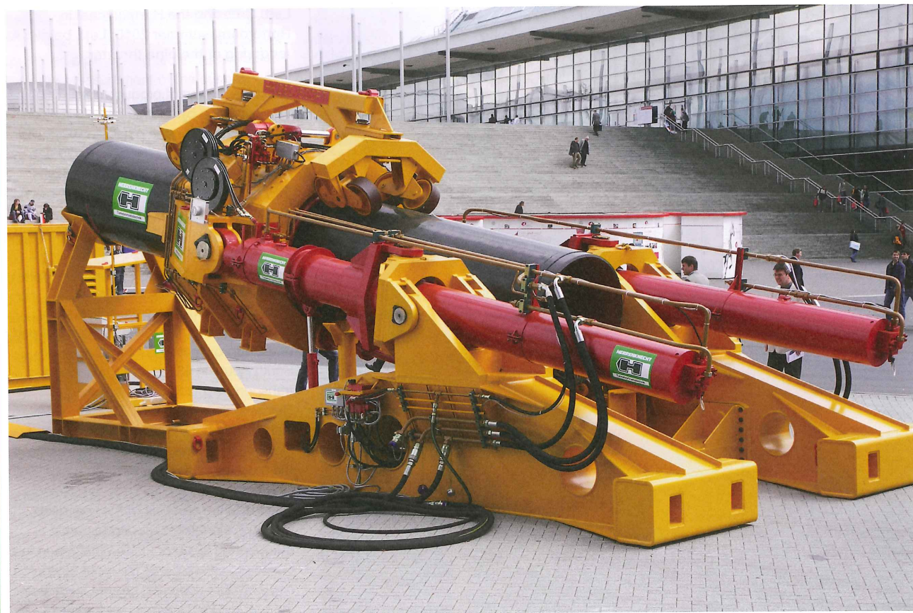
Above: The pipe thruster on display at Messe Hanover—where it was first launched by Herrenknecht
