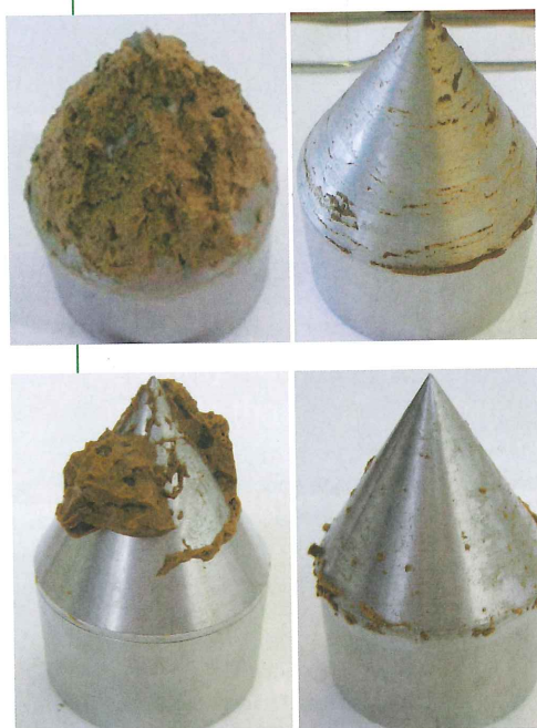
Above, top: Figure 8, Adherences to the test cone for water (left) and 1mol NaCl (right); Above, bottom: figure 9, Application of electro-osmosis to reduce clogging in laboratory on a pure smectite
