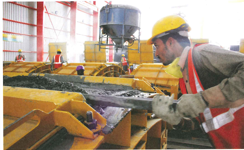
Above: The steel CBE moulds were built to French standards
