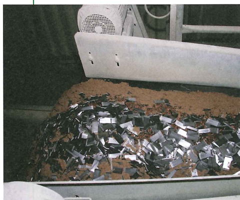
Below: Batching plant material loading belt carrying aggregate and fibres
