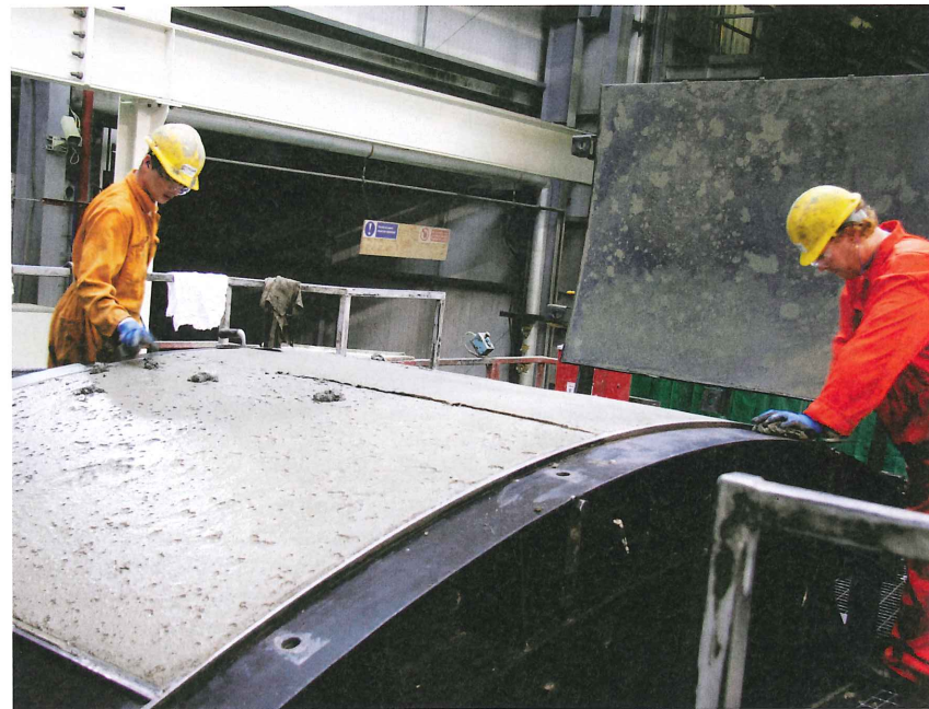
Right: Finishing the extrados face of a segment in the mould
