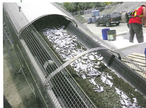
Above: Dramix fibres on their way to the mixer at the Costa Rica segment casting plant for Seli's hydropower tunnel contracts in Panama
