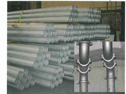
Above: Ground ends to Victaulic pipes avoid the use of welding during installation and are easily connected
