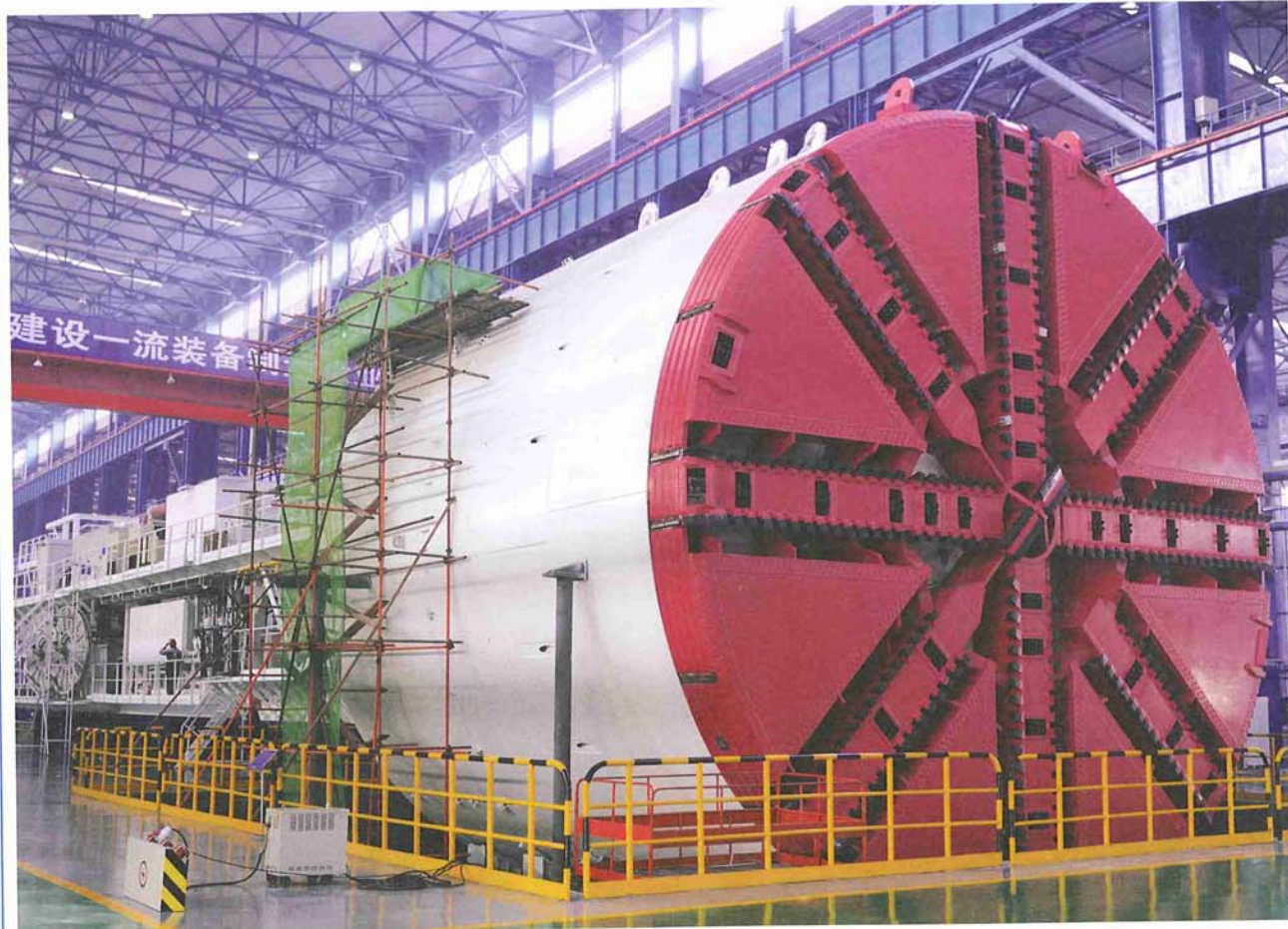
Above: NFM/NHI 11.97m diameter slurry TBM for Tianjin's interconnection tunnel
