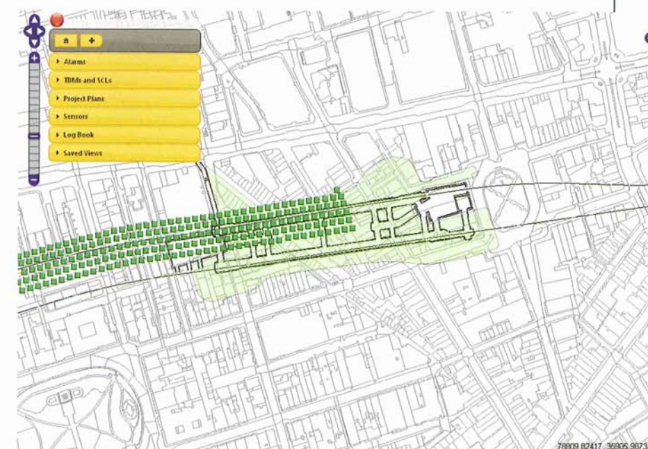
Above: Display image of sensor points in itmsoil's Argus software with integrated GIS
