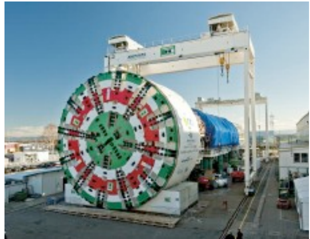
Above: The world's largest EPB TBM assembled in the Herrenknecht yard at 15.62m diameter and 130m length
