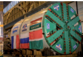
Soft ground TBM
