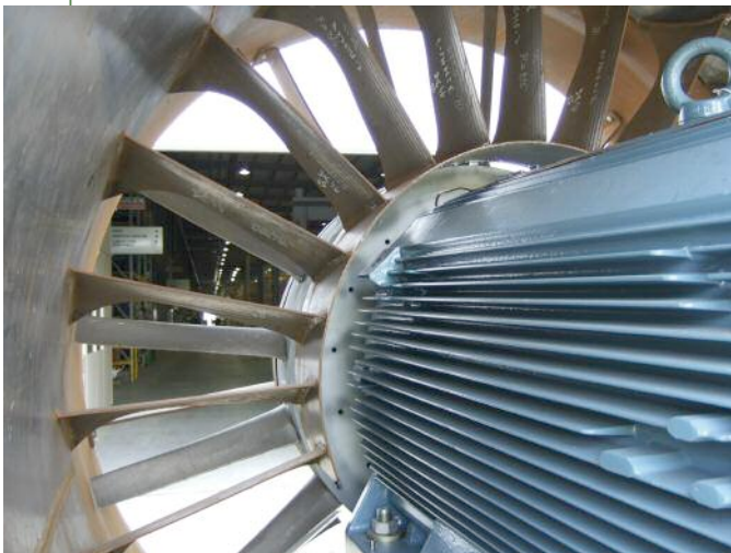
Above: A large Flakt Woods axial fan during certification tests
