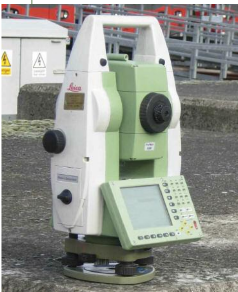
Left: One of the six Leica total stations used for subsidence monitoring surveys
