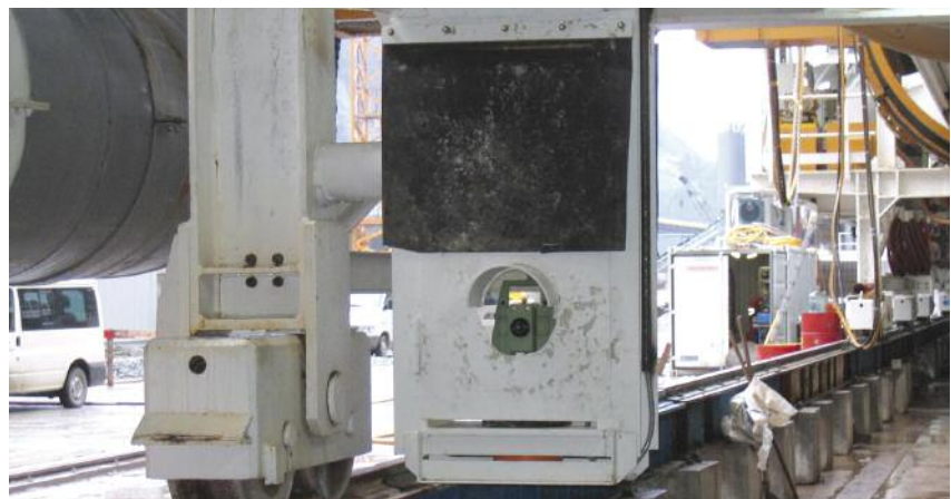
Below: Fig. 1 – The shielded total station used in Gotthard North TBM guidance
