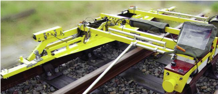
Left, top: The Track Quality Measurement trolley (TQM) for precise checking of rail-track dimensions that may be affected by tunnelling
