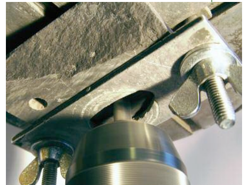
Above: Figure 2 – Outline of the sievers' J miniature drill test to determine Sievers' J-Value (SJ)
