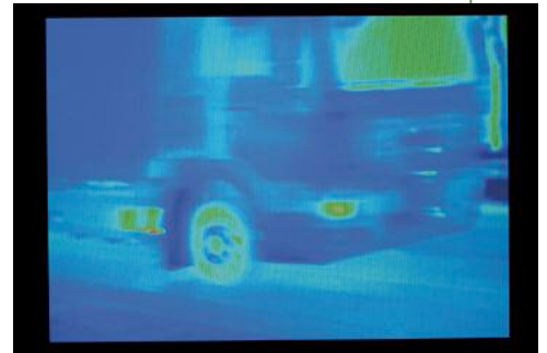
Left: The Vicotec smoke and noxious gas detector from SICK-Maihak Above: Testing the components of Siemens' RFID system to identify hazardous loads Right: Infrared image of a truck before tunnel entry showing hot spots [Siemens press photo]
