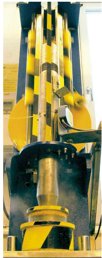
Below: Figure 1 – Outline of the brittleness test used to determine Brittle Value (S 20 ) Right: Brittleness testing for determination of S 20 – close-up of impact weight hitting mortar with rock sample material [Photo: Simon A Hagen]
