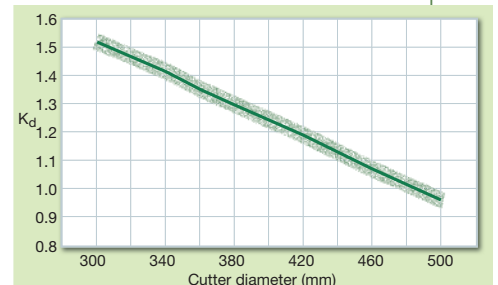
Right, top: Figure 4 – Correction factor for cutter diameter (Salehi – 2007 2 ); Right, bottom: Figure 5 – Correction factor for average cutter spacing (Salehi – 2007 2 )
