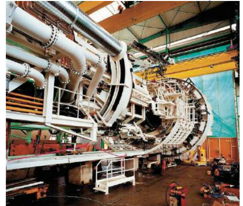
Above: The Asa Herrenknecht TBM with the shield. Note the grouting/probe drill near to crown
